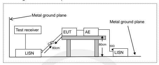
LISN: Line Impedance Stabilization Network
