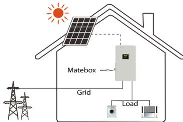
Diagram A: Neutral line and PE line are separated from each other, all loads connect to the EPS (Off-grid) port;
