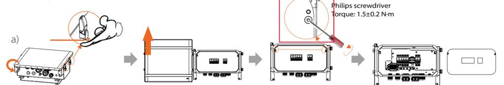
b) Put the matebox on the bracket. Make sure the box is well fixed on the bracket by screwing all nuts tightly.
